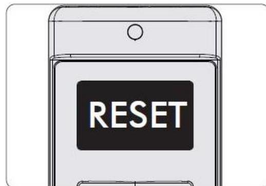
**4** Select the RESET function by pressing the toggle switch.
