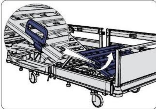
3 Raise the lower leg rest to its full extent by lifting the mattress restraint rail.
