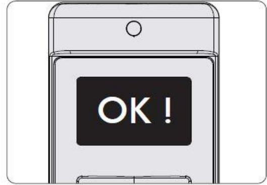
7 The OK ! displayed indicates the successful pre-setting of the intermediate stopping position. The symbol for the intermediate stopping position is then displayed again.
