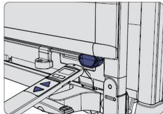
**2** Press the UP and DOWN buttons simultaneously and at the same time hold the top end of the LCD handset briefly against the magnetic unlocking key at the foot end of the bed.
