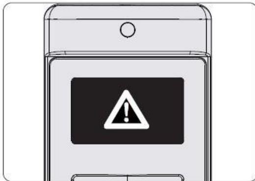
**1** The warning triangle symbol is displayed on the LCD handset. All adjustment options are locked.
