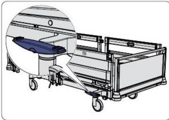
1 The foot lever is located at the foot end of the bed.
